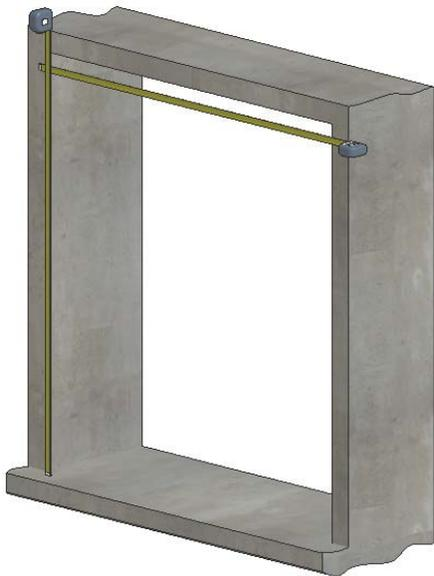
Note: For proper door operation and drainage it must be installed *PLUMB* and *LEVEL*.
